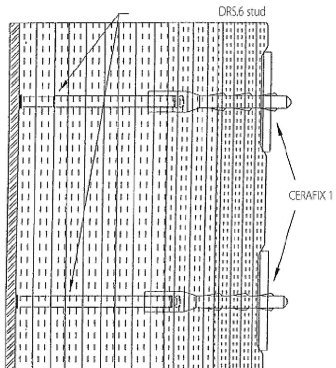
DRS.6 stud is a 6 mm threaded metallic stud that is available in specified lengths. The DRS.6 is available complete with ferrule for stud welding in several alloys (304, 310, 330, 601).
